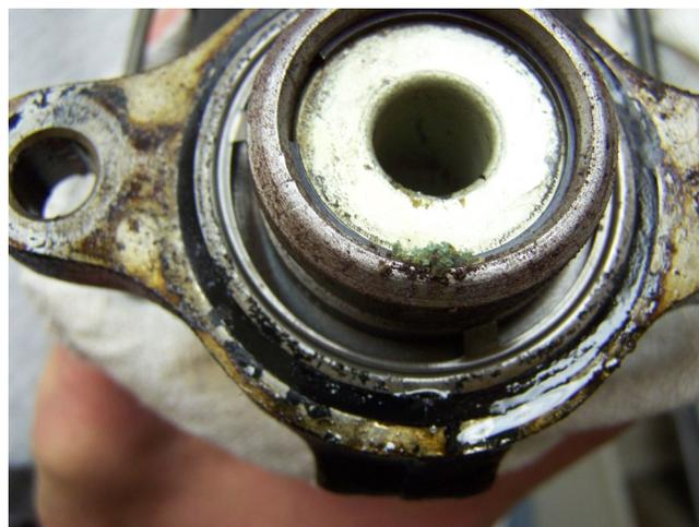
Run DOT 3 (or DOT 4 which is compatible with DOT 3 but with a higher boiling point) only. Space does not allow for all of my arguments and documented problems with DOT 5 silicone fluid here, so let's just suffice with this: DOT 3 is the fluid installed in your car originally, and guess what—it still is today. Keep it fresh and you won't be tearing your brake system down.
